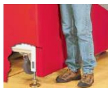
Ratchet Style Front Foot Leveling
